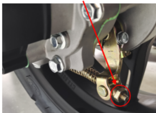
Rear brake cable adjustment nut
