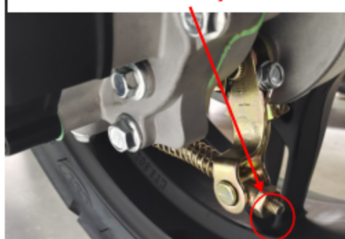
Rear brake cable adjustment nut
